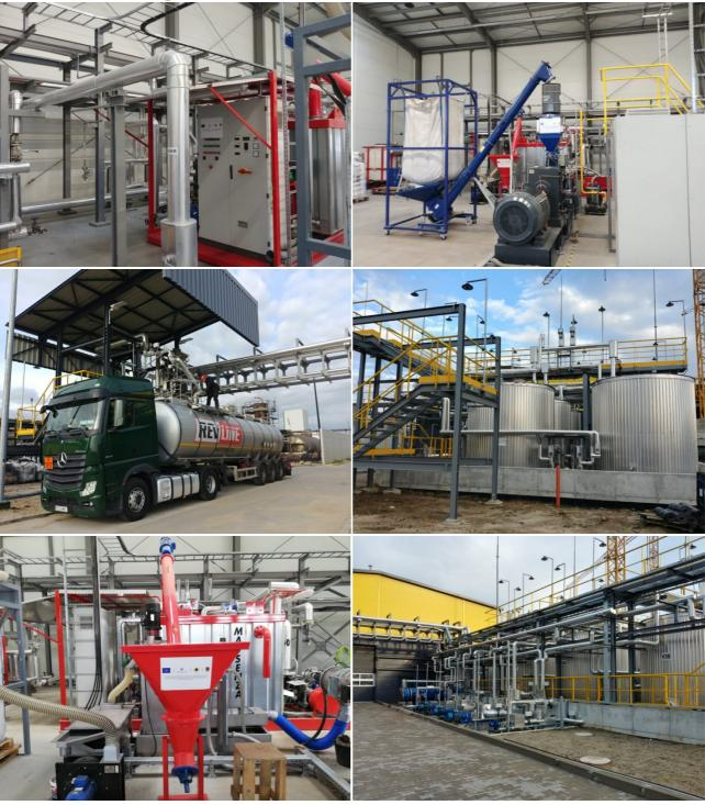
Fig. 9 Pilot installation for the production of asphalt emulsions modified with waste polymer nanostructures
